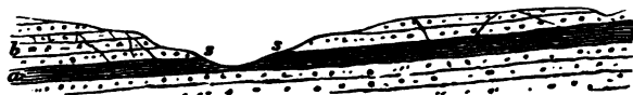
FIG. 46.—Section across a valley to show how the simplest kinds of springs arise.
